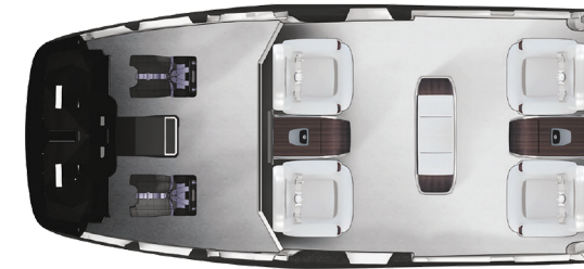
4 - PASSENGER + Foreword & Aft Cabinets + Optional Cabinet + Separation Wall
